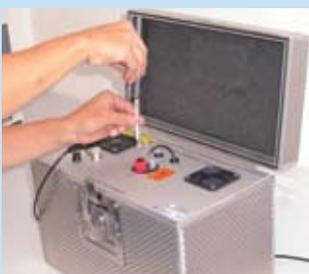
Manual calibration of the mercury analyzer. A known volume of calibration gas is drawn from the calibration device using a gas-tight microsyringe and injected into the analyzer's calibration port.
