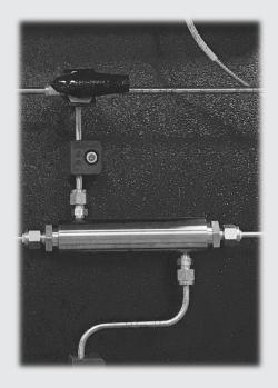
"The Icon Scientific Colour Opacity Analyser is extremely versatile and may be readily re-application engineered by the user in the field. The use of a solid-state spectrometer module avoids the band pass and transmission loss problems associated with optical filters and moving parts such as filter wheels and chopper motor assemblies".
