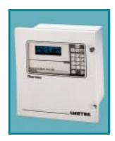
Display: Four-line x 20-character vacuum fluorescent. Displays combinations of oxygen, % or ppm combustibles, time and date, cell temperature, user-programmable text, thermocouple mV or cell mV. Password protection, programmable pressure compensation and context-sensitive help are also provided.
